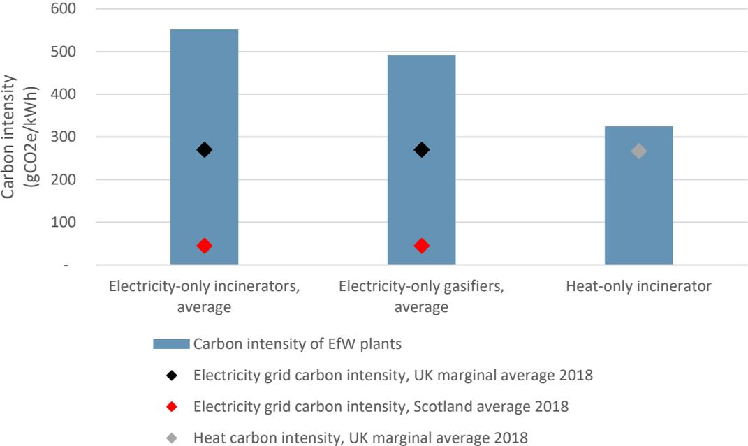
On average, sending one tonne of municipal waste to EfW in Scotland in 2018 emitted 219 kgCO<sub>2</sub>e/t, which is 15% less than sending it to landfill (Figure 2). The results for greenhouse gas emissions per tonne of waste differ considerably for each plant.
