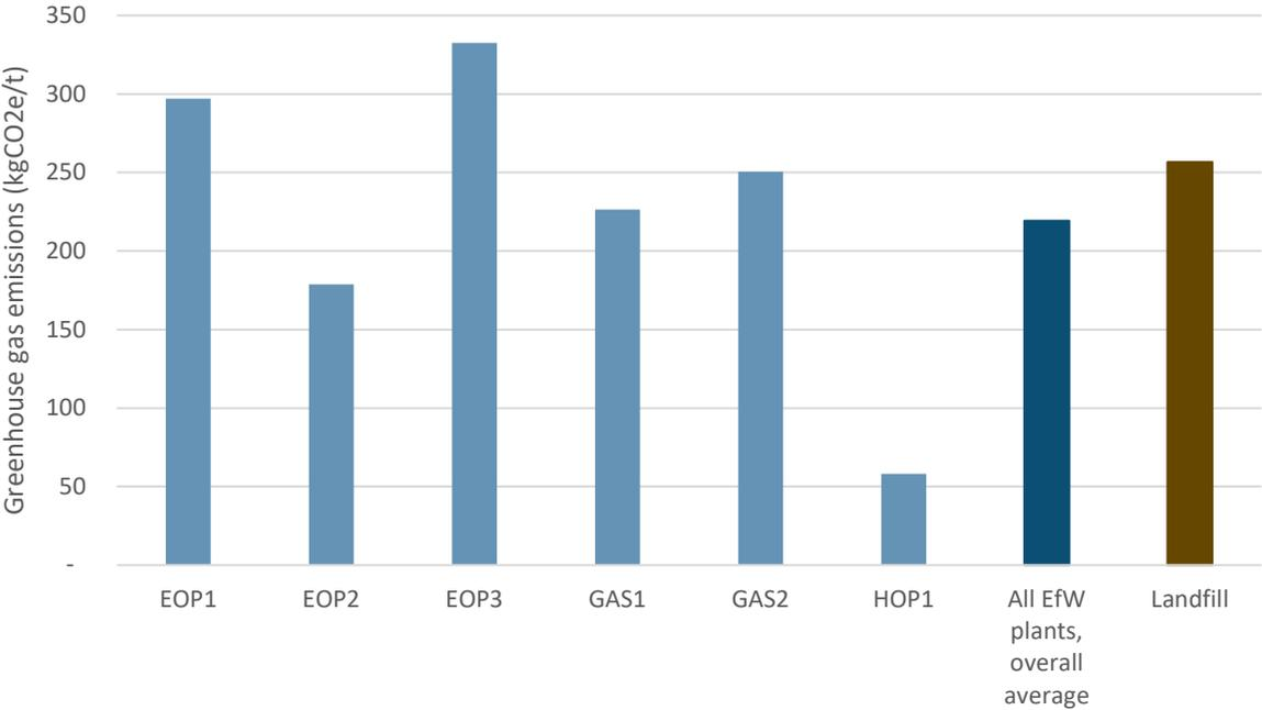
HOP1, the heat-only EfW plant, has lower greenhouse gas emissions per tonne than the other EfW plants because heat-only plants run at a higher efficiency (usually around 50%, compared to 25%). This means much more energy generation can be displaced – reducing the net greenhouse gas emissions per tonne.
