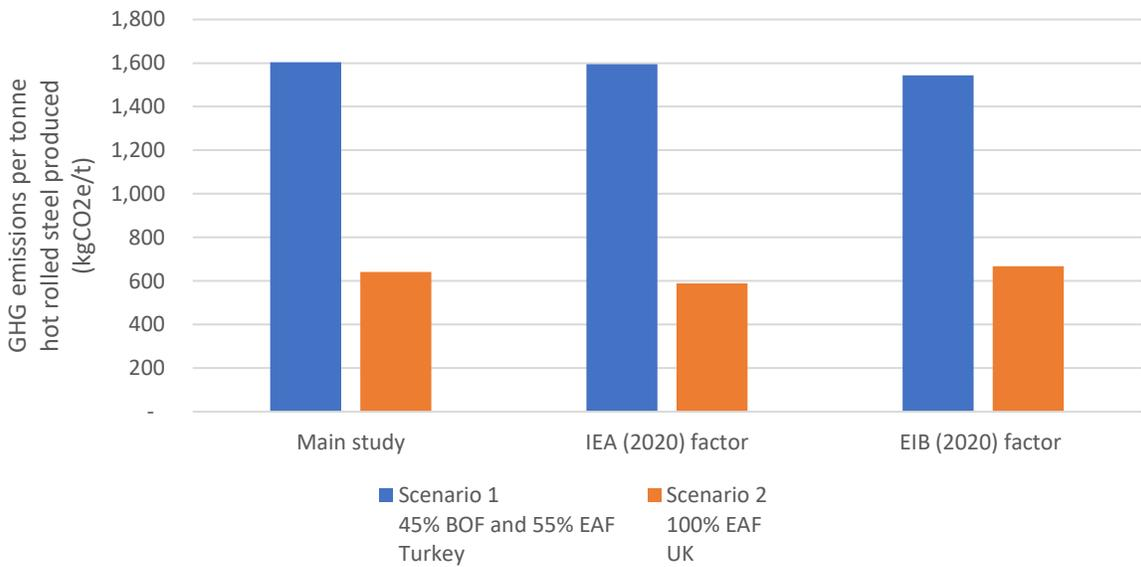
**Figure 1. Effect of changing electricity grid carbon intensity factors on GHG emissions per tonne of hot rolled steel produced**
